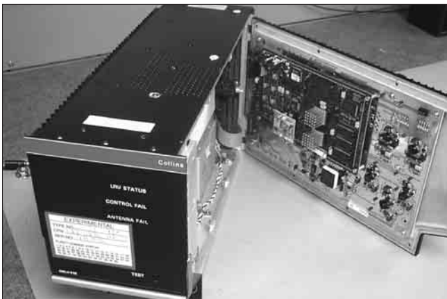
The Loran receiver and interface boards in the MMR. The interface card is mounted on the MMR door and supports the receiver card. The receiver card measures 100 × 160 millimeters.
