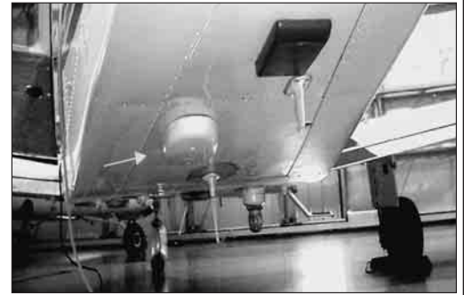
Housed in a certified ADF radome, the H-field antenna was mounted under the fuselage of a Piper Saratoga.
