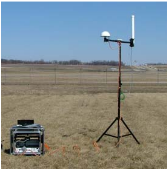
Figure 4b. Locus' ASF generation system in operation at the Jacksonville Craig Airport during the March 2004 flight trials. The tripod is used to support Loran H-field (left), GPS (center), and Loran e-field (right) antennas.
