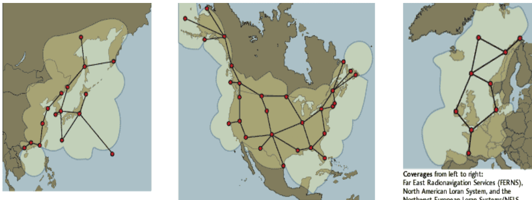
Figure 1. Loran-C map of coverage from left to right: coverage provided by FERNS, North America Loran and NELS (Courtesy of Megapulse, Inc.) [2].
