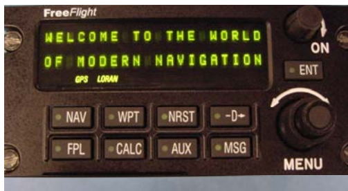
Figure 2a. Face plate of the original 2101 system used in the two-unit prototype. FFS developed software to control the SatMate 1030 and display Loran information.
