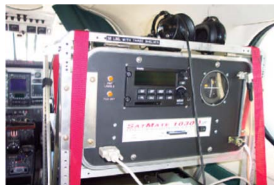
Figure 1. The first GPS/Loran prototype system as rack-mounted and strapped down in the AEC's King Air, C-90SE twin turboprop. In this prototype, a course deviation indicator (CDI) was added and is in the upper right of the front panel. The 2101 is top center and the
